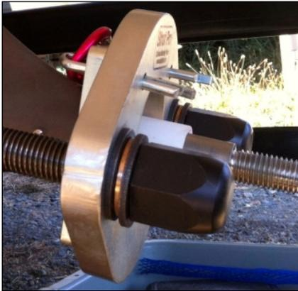
The tool is now installed and you are about to remove the bearing. Apply equal pressure to both threaded rods. If you are using a  $\frac{3}{4}$ " ratchet then about three pulls on one side then switch.
